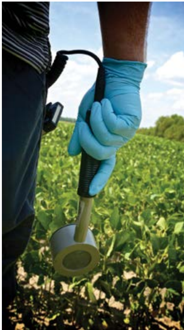
Photo: Person holding a radiation detector conducting radiation survey of a field
