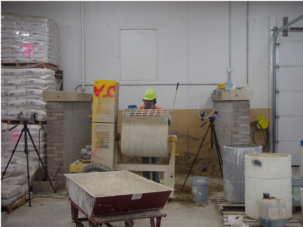
Figure 1 - Mortar Mixer Inside Training Center, Showing Area Sampler Locations
