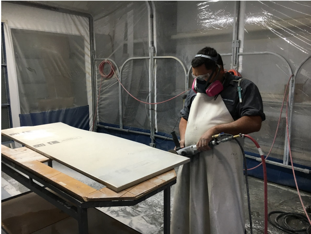
Figure 3 – A worker using a handheld pneumatic wet grinder with a diamond grinding cup wheel inside the dust control booth. Photo by NIOSH
