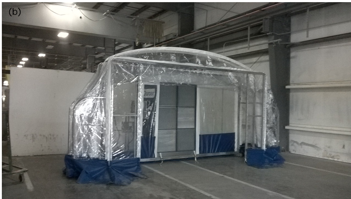
Figure 2 – Duroair dust control booth (a) fully extended; (b) retracted. Photo by NIOSH
