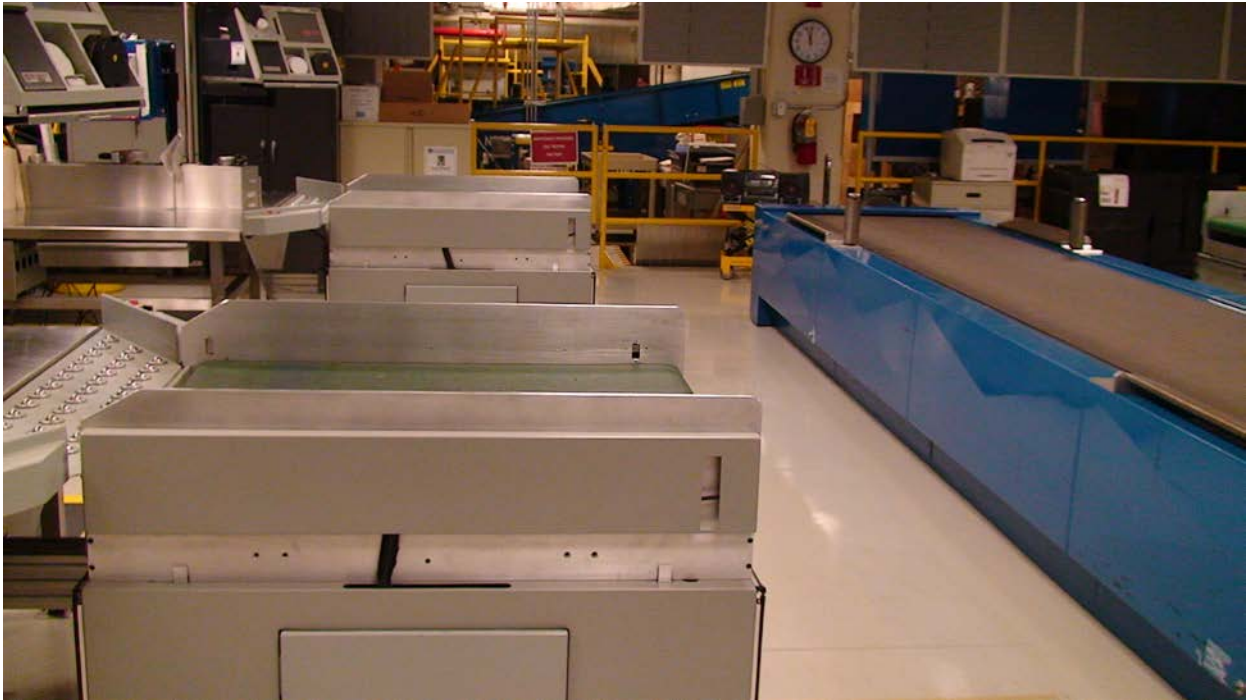
Figure 2. The Bagwell Oversize Baggage (BOB) Moving System was evaluated in the study
