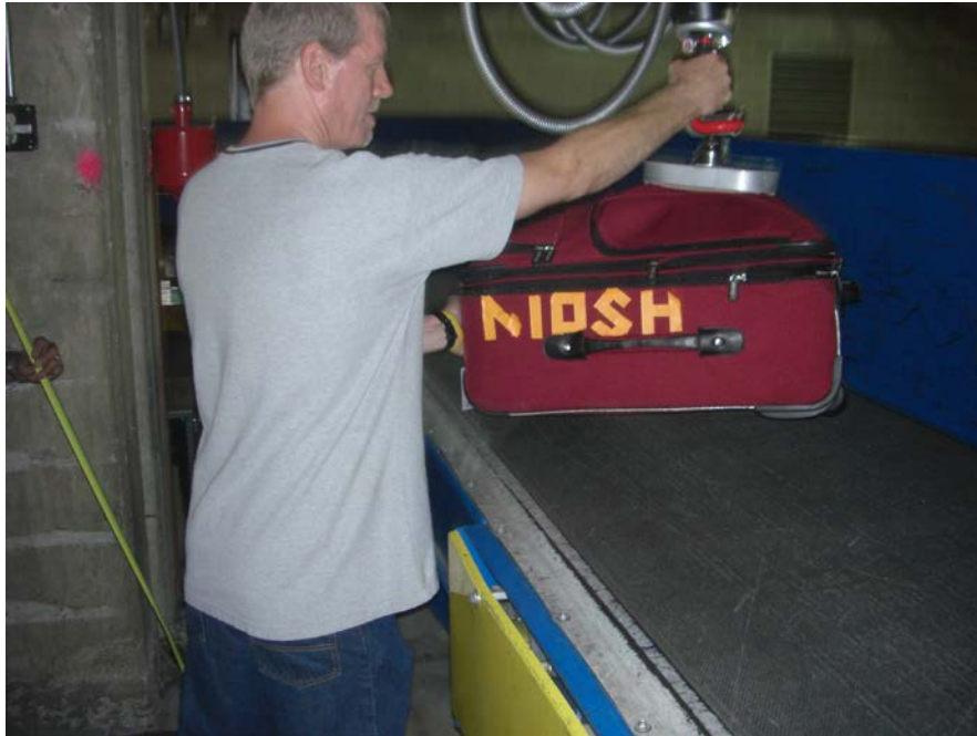
Figure 3. On site mock-up testing was used for measuring hand and thumb forces required for using the Vaculex ® TP system
