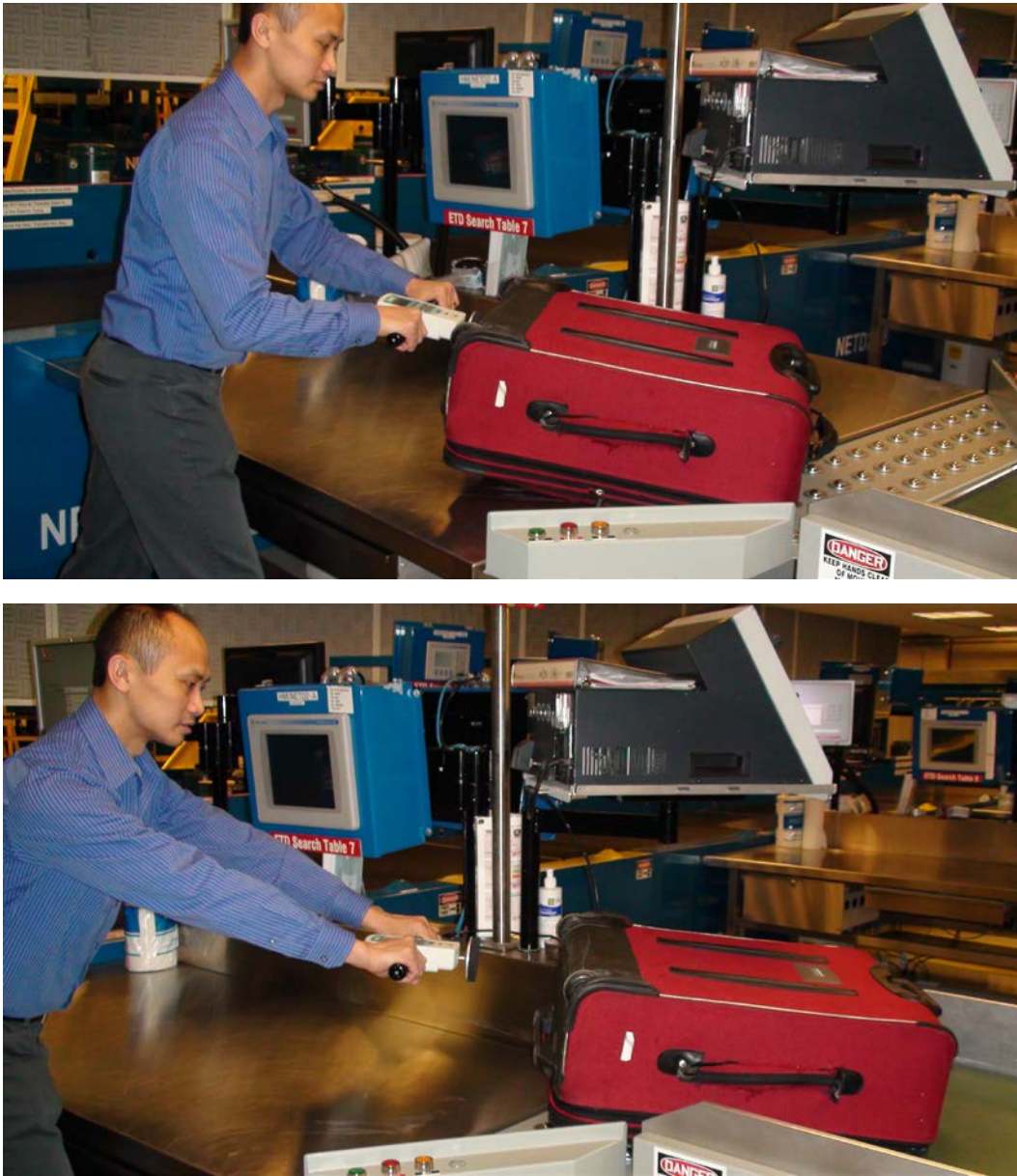
Figure 4. On site mock-up testing was used for estimating hand forces required for pushing a bag to the BOB moving system (upper and lower pictures show the start and end of the pushing task)
