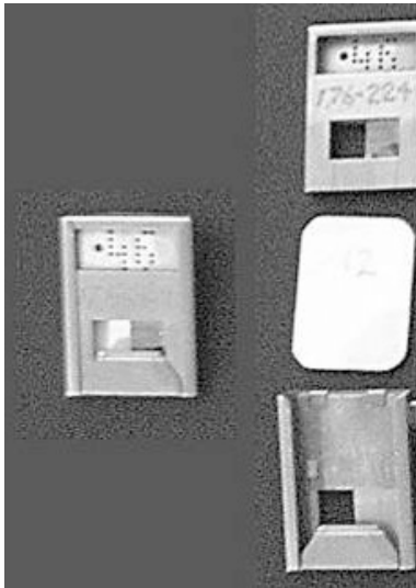
Figure 6-2. ORNL-style film badge (including brass filter).
