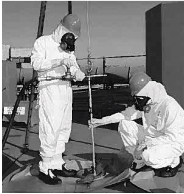
Figure 2-3. SRS workers measuring the level of waste in a tank.
