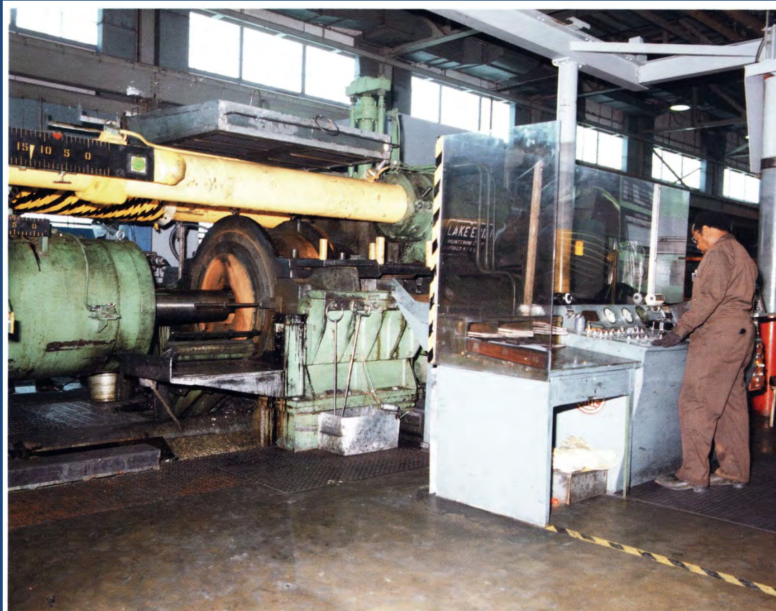
A composite billet of uranium-aluminum alloy encased in aluminum enters extrusion press at the left and emerges at far right.
