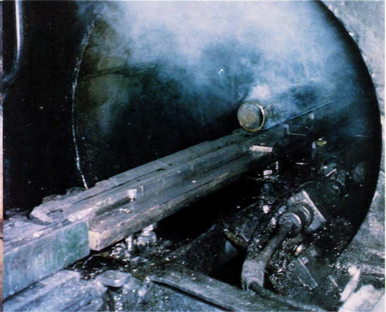
Fuel tube emerging from die.
