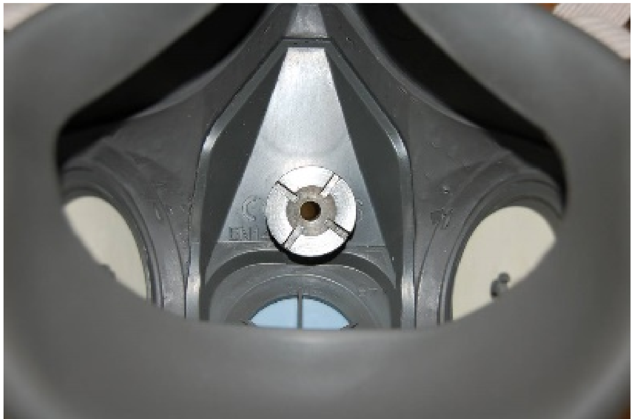
Figure 8: Interior View of a Probed Sample Respirator
