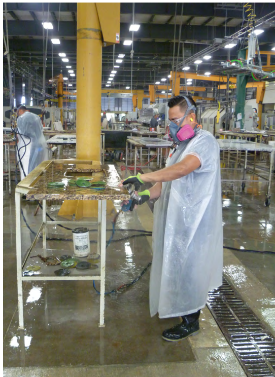
Figure 2. Employee using a hand polishing tool outfitted with a water spray. Photo by NIOSH.
