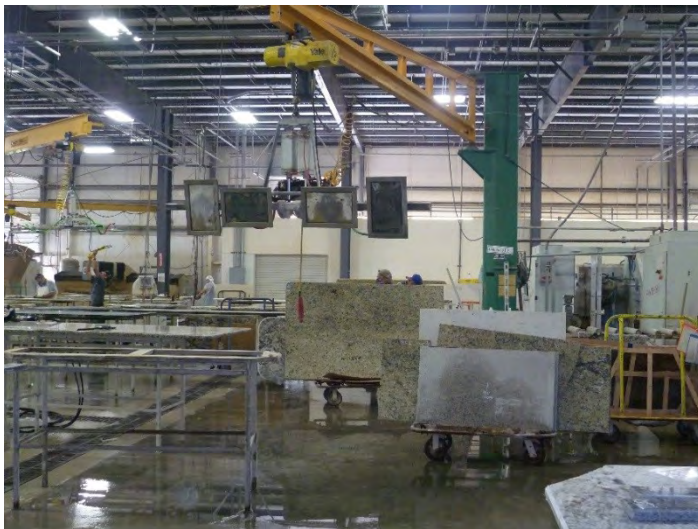
Figure 7. Slab lifter attached to overhead crane. Photo by NIOSH.
