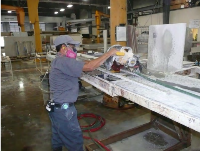
Figure 3. Photo of a lamination employee making a cut with a miter saw. Photo by NIOSH.
