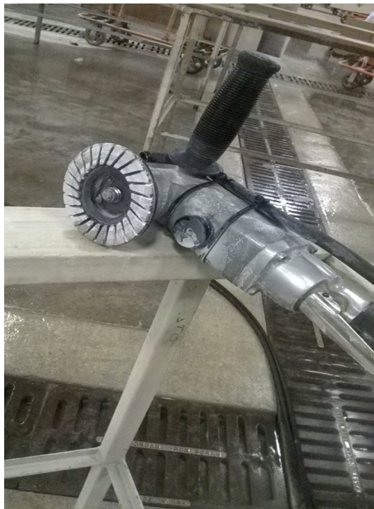
Figure 1. Photo of a pneumatic wet grinder equipped with a diamond cup wheel and a water spray used in the polishing area. Photo by NIOSH.
