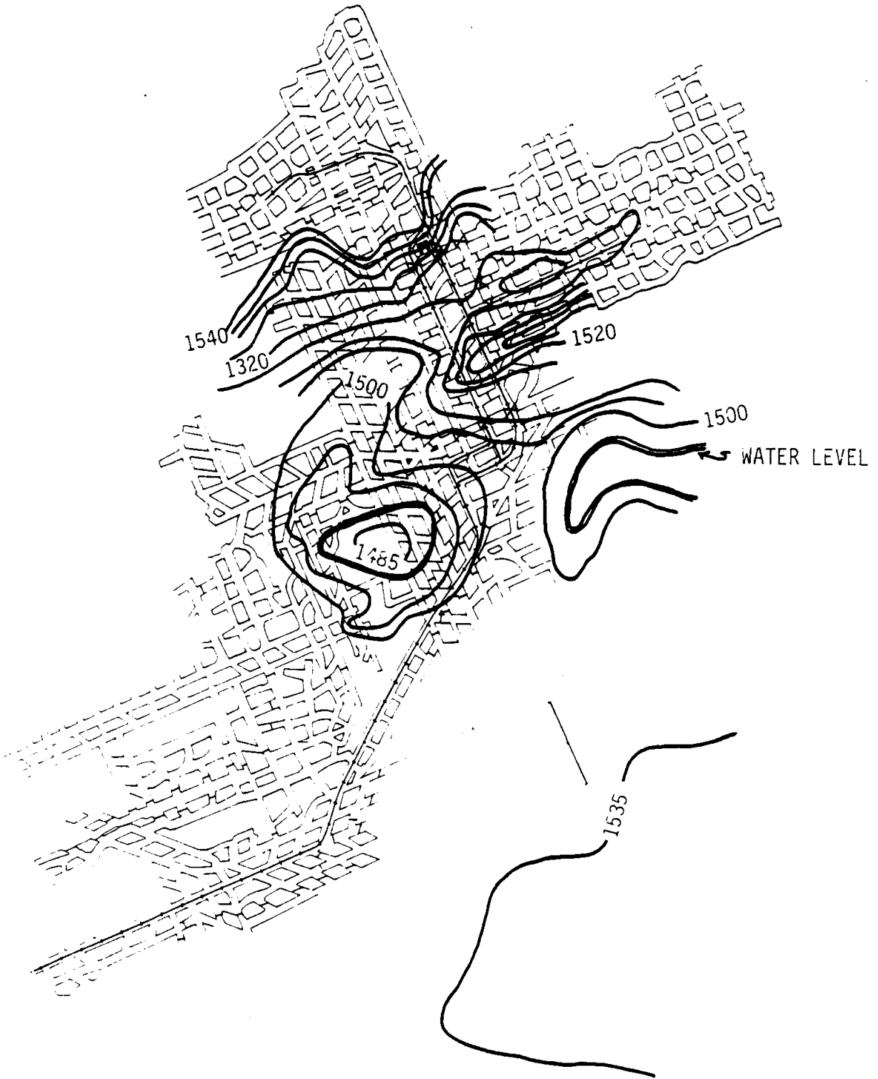
(b) STRUCTURE CONTOURS OF THE SEAM
