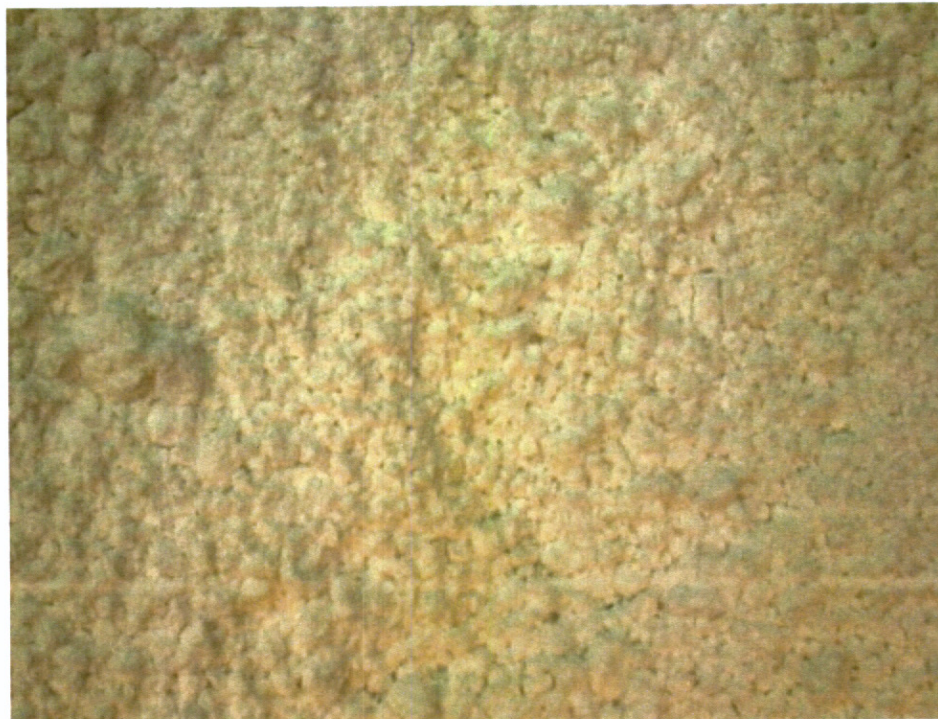
Figure 23. NIEHS nonasbestiform tremolite sample.
