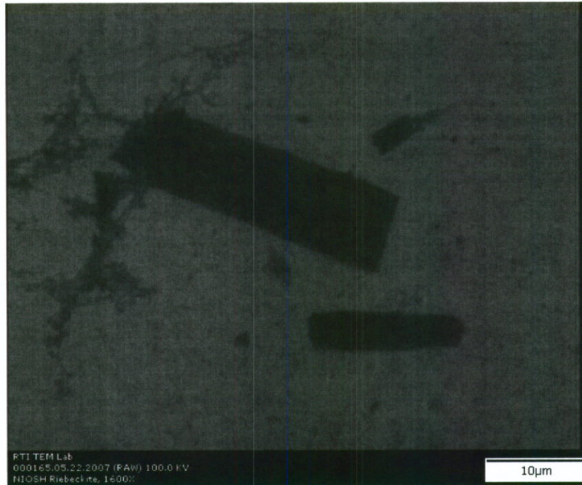
Figure 40. TEM photograph of Riebeckite preparation. 1600X
