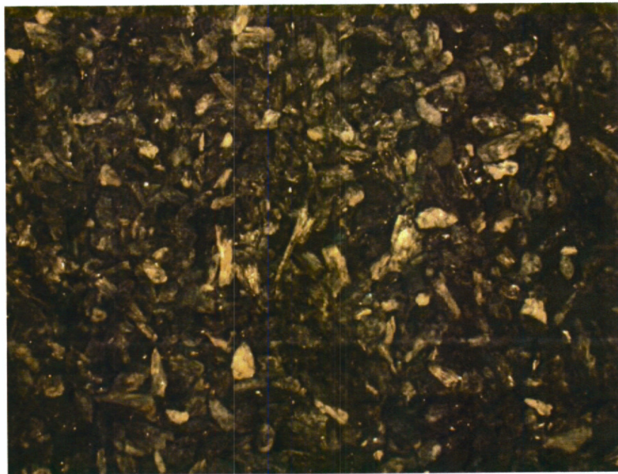
Figure 19. Cummingtonite sample following hydraulic crushing.
