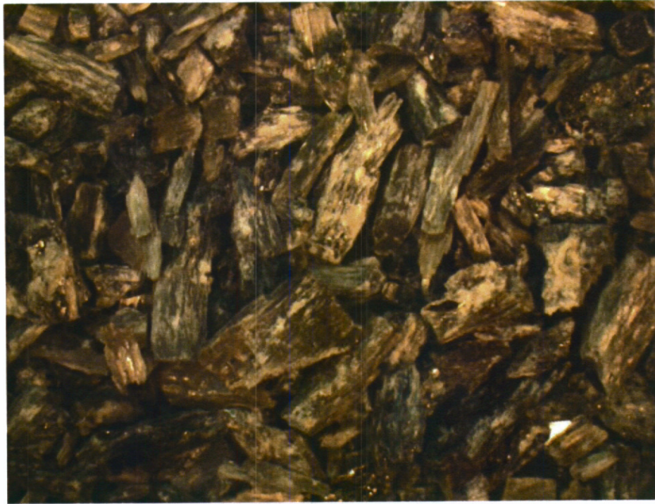
Figure 22. Anthophyllite sample following hydraulic crushing.
