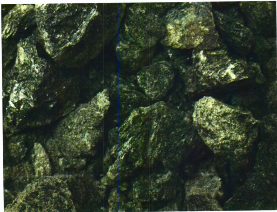
Figure 21. Grunerite sample following hydraulic crushing.
