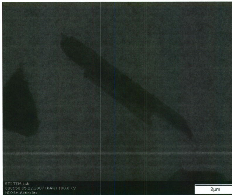
Figure 37. TEM photograph of Actinolite preparation. 8000X
