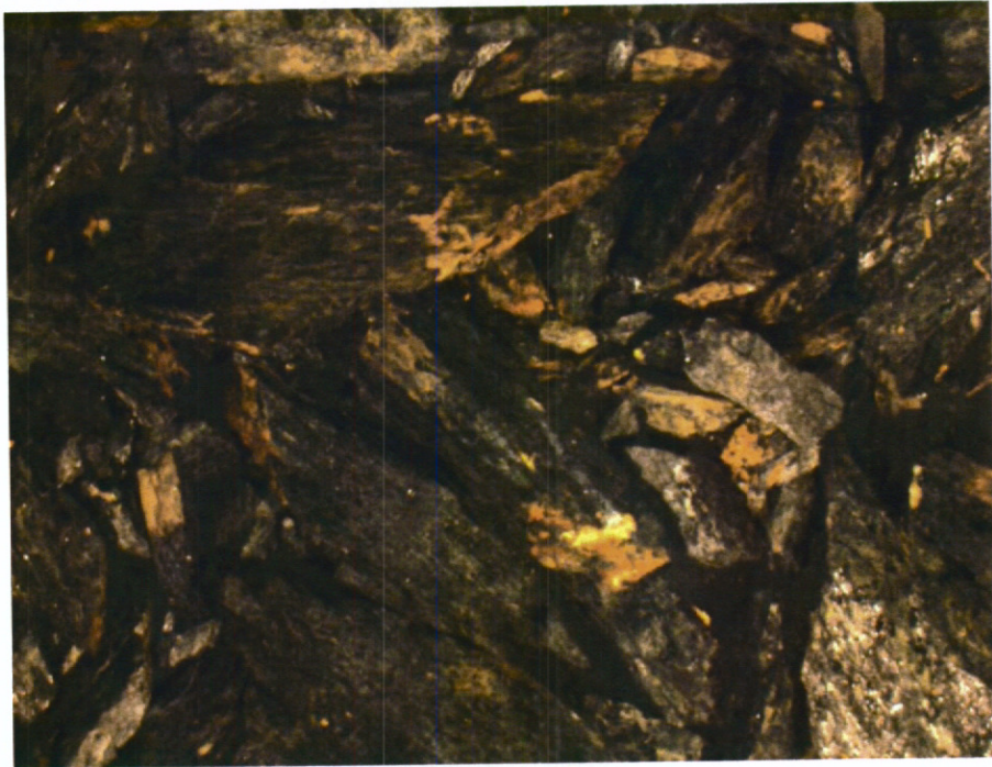
Figure 20. Riebekite sample following hydraulic crushing.
