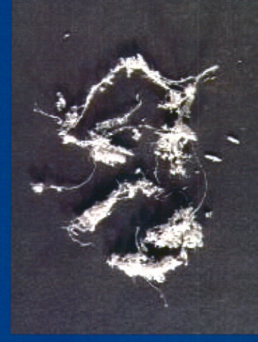
HSE Reference Tremolite Asbestos
