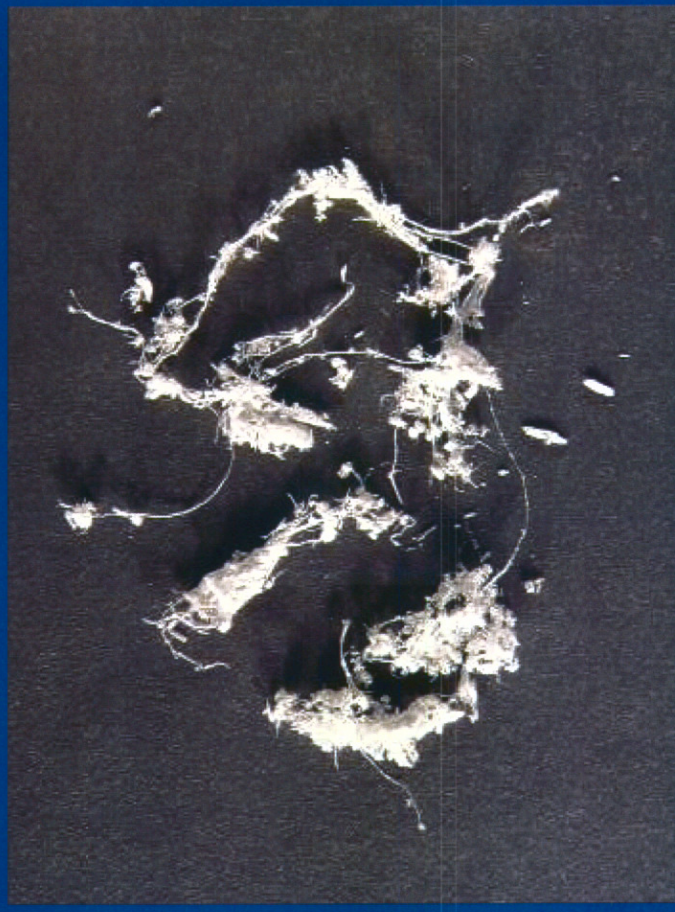
HSE Reference Tremolite Asbestos
