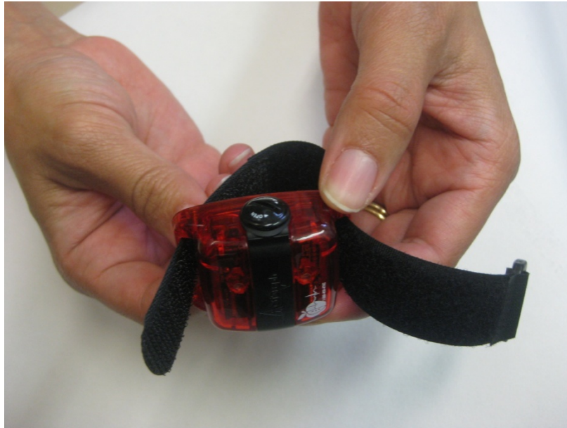
Exhibit 3-11. Threading the wrist strap through the PAM
