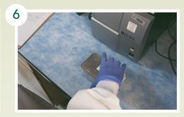
Once properly sealed, the plates are ready for incubation. Stack the plates and sandwich them in between two empty plates.
