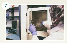
Make sure the temperature in the incubator is within ±2°C of 37°C and that the fan works to distribute the heat evenly. Place the plates in the center of the incubator. Keep the plates incubated for approximately 42 hours.
