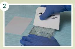
Use a flat object to press the sealing membrane down to remove any air.
