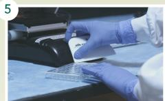
Apply additional manual sealing to prevent leakage and improve precision. Use a flat object to press the sealing membrane down and to carefully seal all edges and corners.
