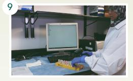
Scan the sample ID's for the unknown samples into Notepad in the same sequence as they were diluted. Return the sample vials to the freezer.
