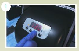
Pre-set the heat sealer to 130°C. Note: if a heat sealer is not available, review steps in the training manual for manual sealing.
