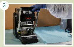
Once the temperature is stable, place a piece of aluminum foil on top of the sealing membrane. Place the plate on the holder and apply heat for 5 sec.
