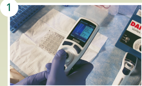
1 Set the volume of a single-channel electronic pipette (20-300 \mu L) with the repetitive pipetting function to 50 \mu L.
